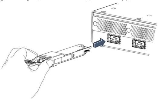
5. Press firmly on the front of the transceiver module with your thumb to fully seat the transceiver in the module's transceiver socket (see the below figure).
