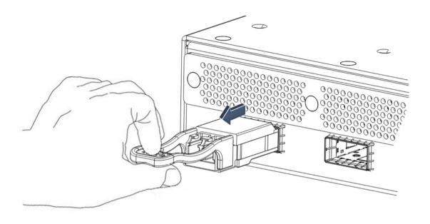
Figure 2. Removing the QSFP-DD Transceiver Module
